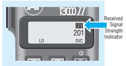
If the Service Indicator is on continuously, your radio has access to a trunking network and is ready to make or accept calls. If it is blinking, your radio does not currently have access to a network. It may be attempting to find a site it is authorised to use, or it may be out of range of a network signal.
