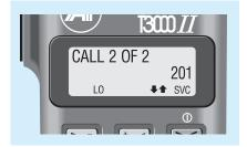
As calls are received and queued, the display shows CALL X OF Y where Y is the total number of calls presently queued, and X is the position of the current call in the sequence. The first call is always displayed until you scroll through the queue. The identity of the caller (a number or label) and their status message (if sent) are also displayed.
