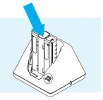
4. Tilt the battery back against the contacts until it snaps into place.
