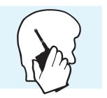
the radio operates normally. Lift it to about 15 cm from your face with the speaker beside your ear and the bottom of the radio beside your mouth as shown. Press and hold the PTT key each time you speak, as described above.
