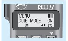
To initiate Quiet mode, use the Menu to set the QUIET MODE option  $ON^5$ . (This feature can also be set by using a dialling sequence. For more information, see Appendix IV, "Common Dialling Functions".)
