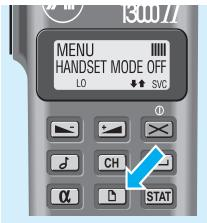
Use the cursor keys to move between menu options. Most menu options have an ON and OFF setting. To change the current setting, press the Enter ( $\leftarrow$ ) key. To leave the menu options and return to normal operation press either the Menu (**b**) key again or the Clear (>) key.
