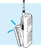
3. Place the battery in the charger pocket with the four silver contacts to the back. Lean the top forward as far as you can to seat the battery properly.
